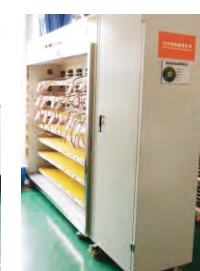
LED Controller Aging Testing Equipment
