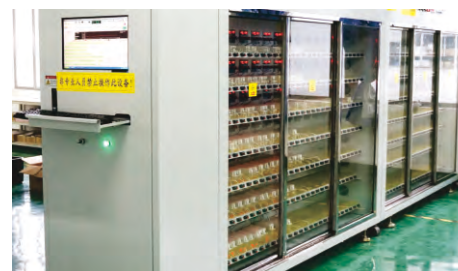
LED Driver Aging Testing Equipment
